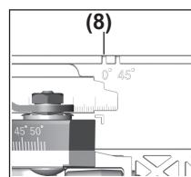
Use only cut marks (8) when making a right-angled cut and a  $45^\circ$  cut with the guide rail.
