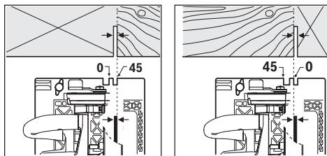
The  $0^\circ$  cut mark (9) indicates the position of the saw blade when making a right-angled cut. The  $45^\circ$  cut mark (8) indicates the position of the saw blade when making a  $45^\circ$  cut. For a precise cut, place the circular saw against the work-piece as shown in the figure. We recommend making a test cut.
