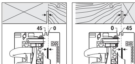
The  $0^\circ$  cut mark (8) indicates the position of the saw blade when making a right-angled cut. The  $45^\circ$  cut mark (9) indicates the position of the saw blade when making a  $45^\circ$  cut. For a precise cut, place the circular saw against the work-piece as shown in the figure. We recommend making a test cut.
